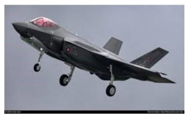
Unlike earlier generation fighter jets, the Lightning is designed to carry its weaponry internally, decreasing drag and its radar signature.
