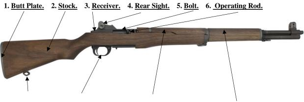
7. Butt Swivel. 8. Trigger Guard. 9. Rear Hand Guard. 10. Front Hand Guard.
