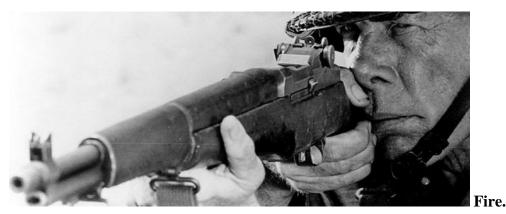
U. S. rifle, caliber .30, Ml. (1) Fully loaded with clips of ball ammunition or with blank ammunition and blank adapter. Squeeze the trigger for each shot. When the eighth shot has been fired, the clip will be ejected automatically and the bolt will remain open for the insertion of a new clip.
